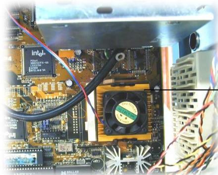
*The CPU chip inside a personal computer is sometimes a bit tricky to spot. It is large and often has its own cooling fan sitting on top.*
